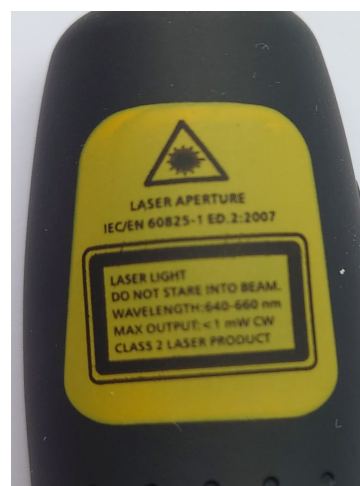
Fig 3. The labelling of the laser used in the experiment
